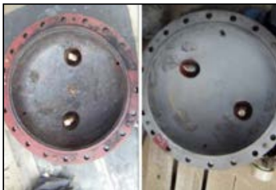
Removal of coal tar epoxy costing
